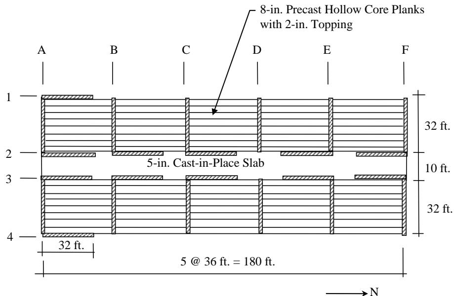
Figure 3-2 Plan view of typical multistory reinforced masonry shear wall building configuration (design for 12-story SDC D<sub>max</sub> shown).
