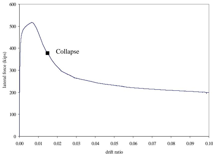
Figure 3-10      Pushover curve for the 2-story, high axial load, SDC D<sub>max</sub> archetype.
