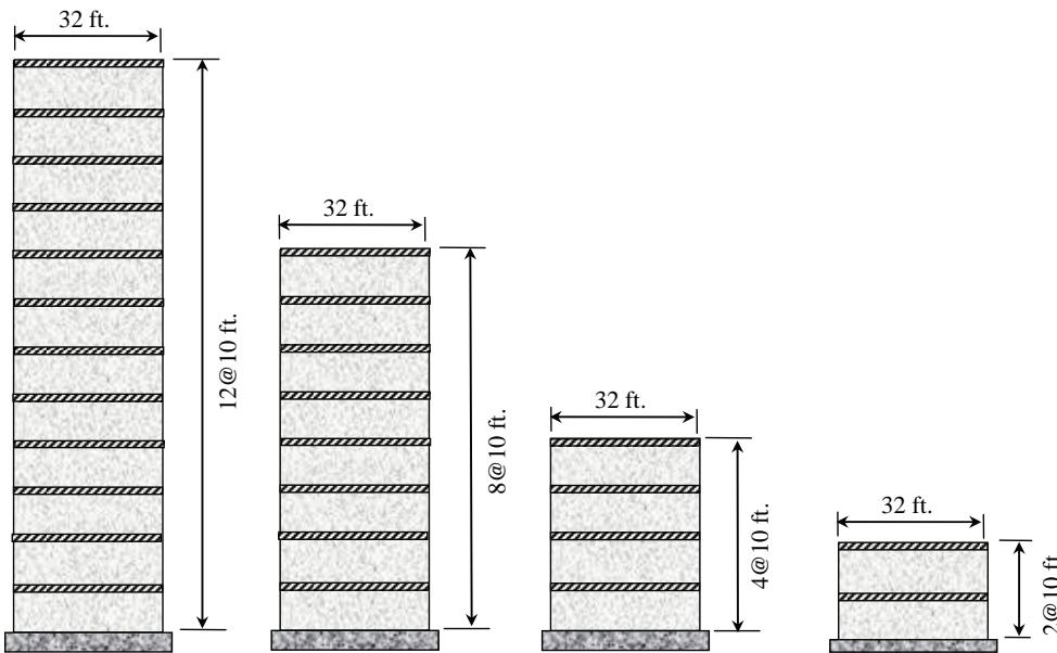
Figure 3-3 Dimensions of multistory reinforced masonry shear walls.
