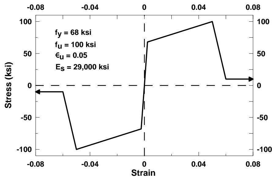
Figure 4-3 Hysteretic material model for reinforcing steel.
