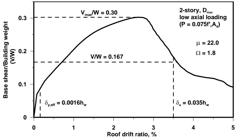
Figure 4-13 Pushover results for the 2-story, low axial load, SDC  $D_{max}$  archetype (ID 12).
