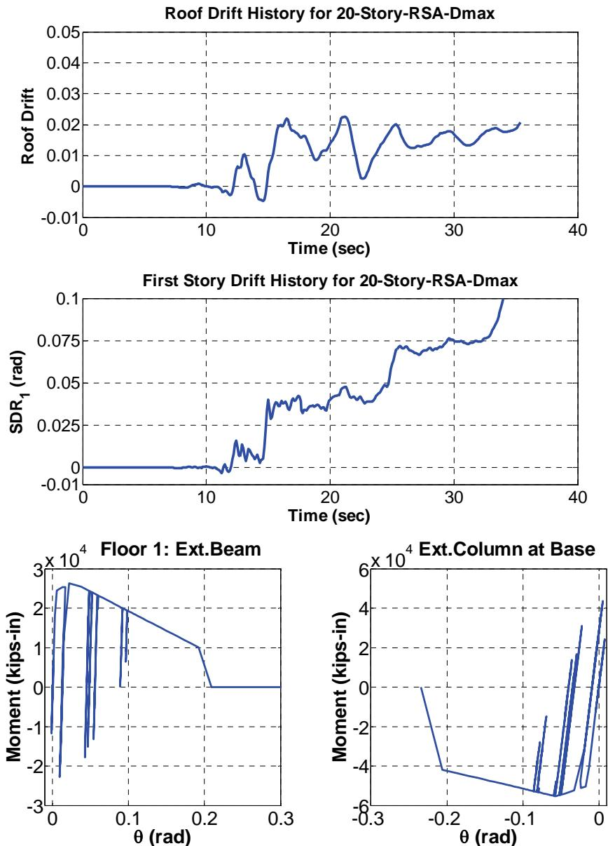
Figure 6-14 Response characteristics of the 20-story, RSA, SDC D<sub>max</sub> archetype at a scale factor of 4.4 (structure collapses).
