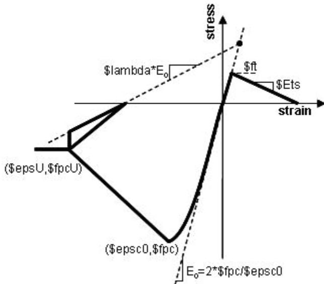
Figure 4-2 Concrete stress-strain behavior model (C02) contained in OpenSees.
