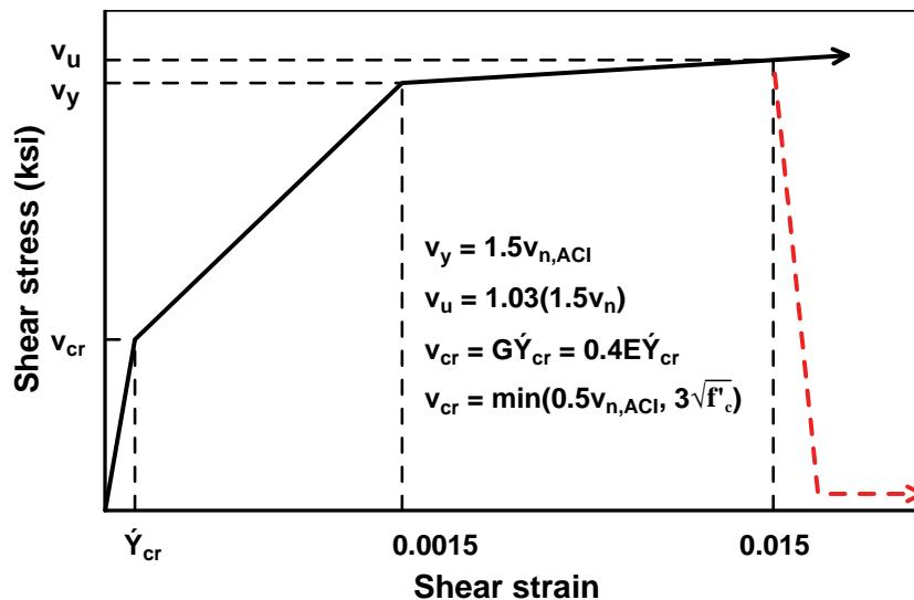
Figure 4-5 Generalized shear model adapted from ASCE/SEI 41-06.
