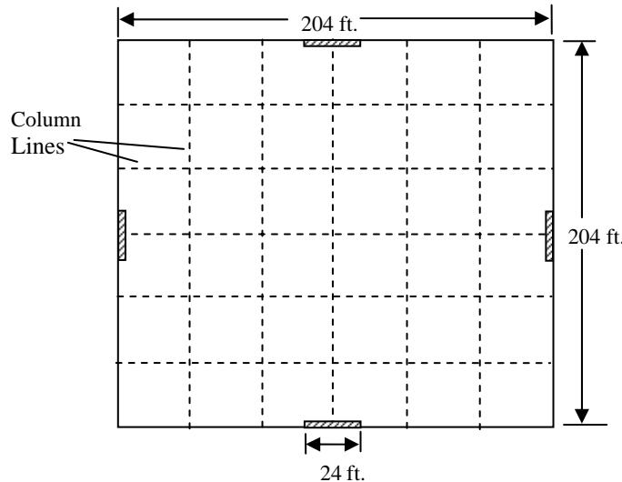
**Figure A-1** Single-story reinforced masonry shear wall building configuration (design for SDC D<sub>max</sub> shown).
