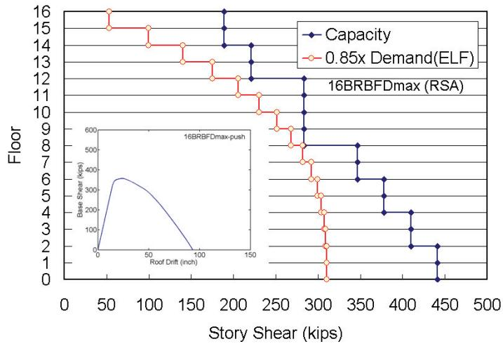
**Figure 5-8** Demand profile of pushover analysis and approximate capacity of archetype 16BRBFD<sub>max</sub> (RSA).
