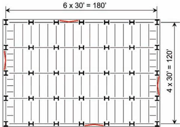
Figure 5-1      Typical plan configuration of special SCBF and BRBF archetypes
