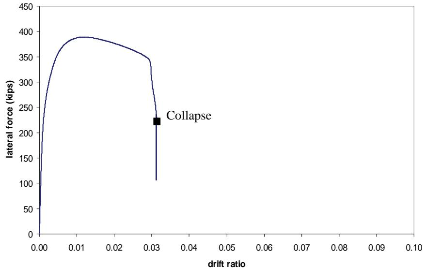
Figure 3-11 Pushover curve for the 12-story, high axial load, SDC D<sub>max</sub> archetype.
