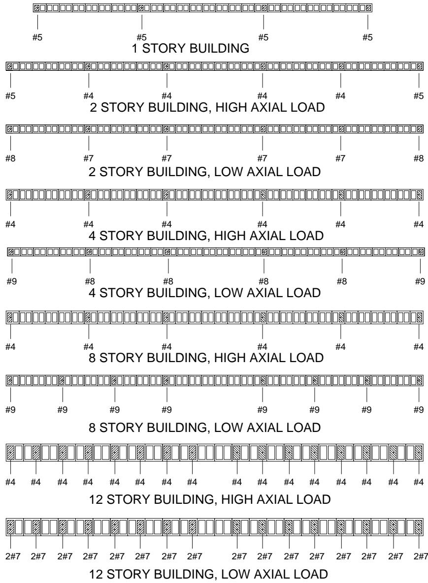
Figure A-5 Plan sections of partially grouted ordinary reinforced masonry shear walls, SDC C<sub>max</sub>.
