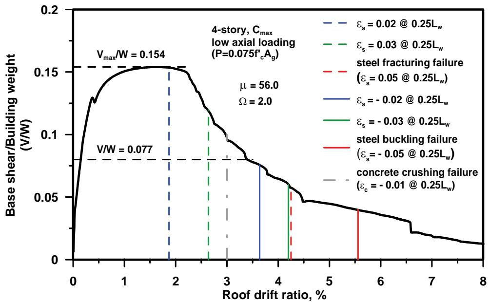
Figure 4-8 Pushover analysis results for the 4-story, low axial load, SDC C<sub>max</sub> archetype (ID 33).
