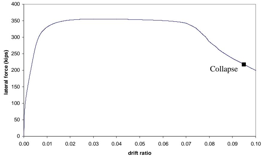
Figure 3-12 Pushover curve for the 12-story, low axial load, SDC D<sub>max</sub> archetype.
