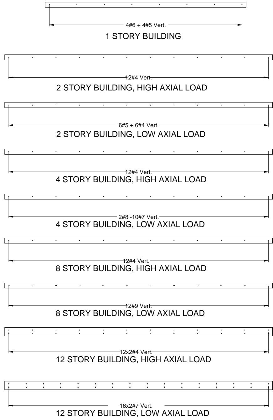
Figure A-4 Plan sections of fully grouted special reinforced masonry shear walls,
