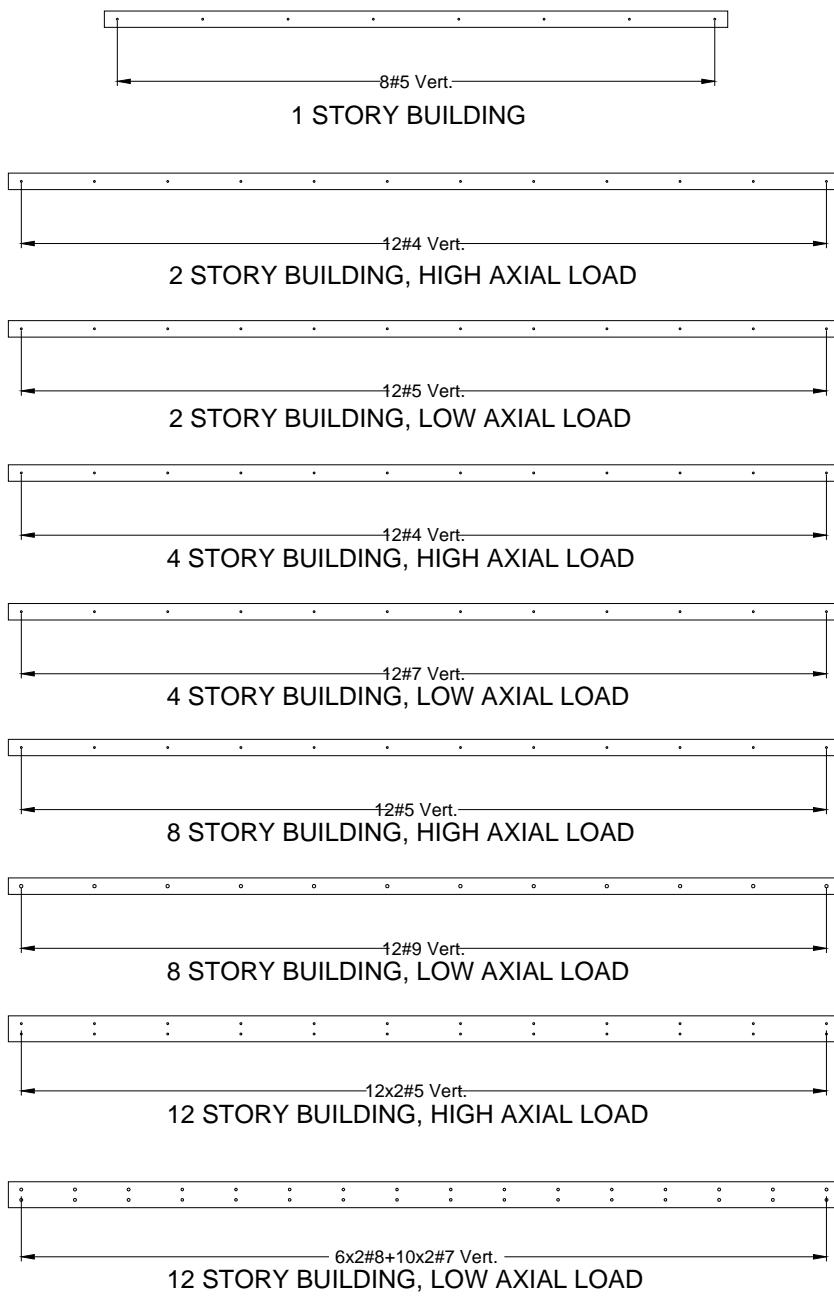
Figure A-3 Plan sections of fully grouted special reinforced masonry shear walls,
