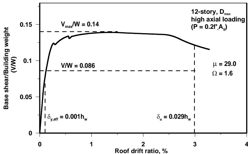
Figure 4-16 Pushover results for the 12-story, high axial load, SDC  $D_{max}$  archetype (ID 5).
