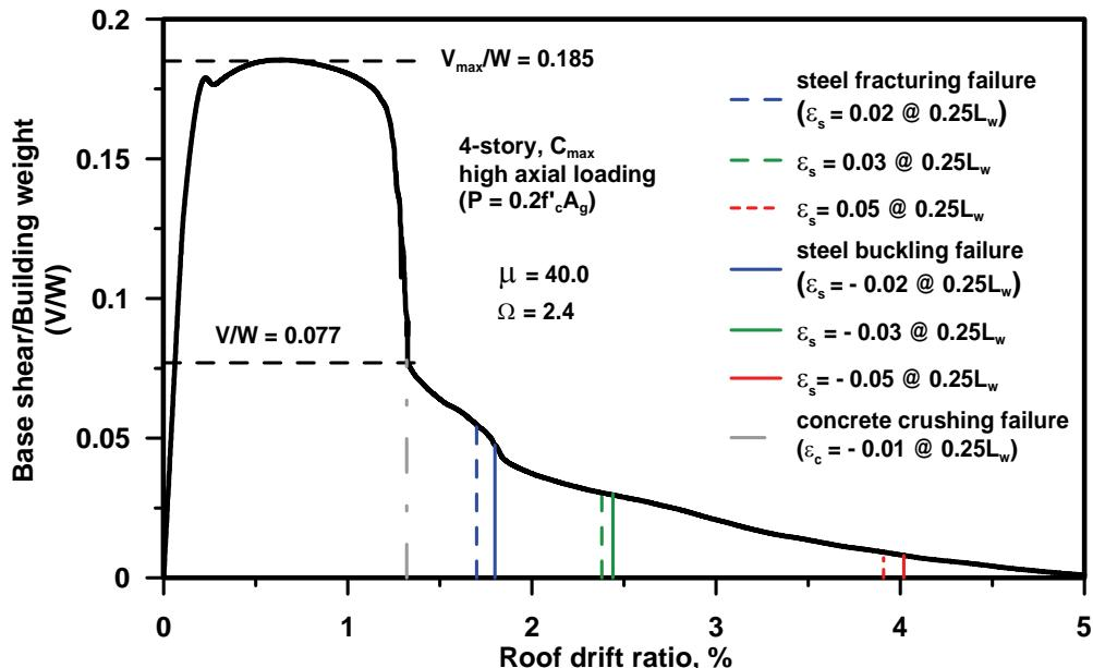
Figure 4-9 Pushover analysis results for the 4-story, high axial load, SDC C<sub>max</sub> archetype (ID 23).
