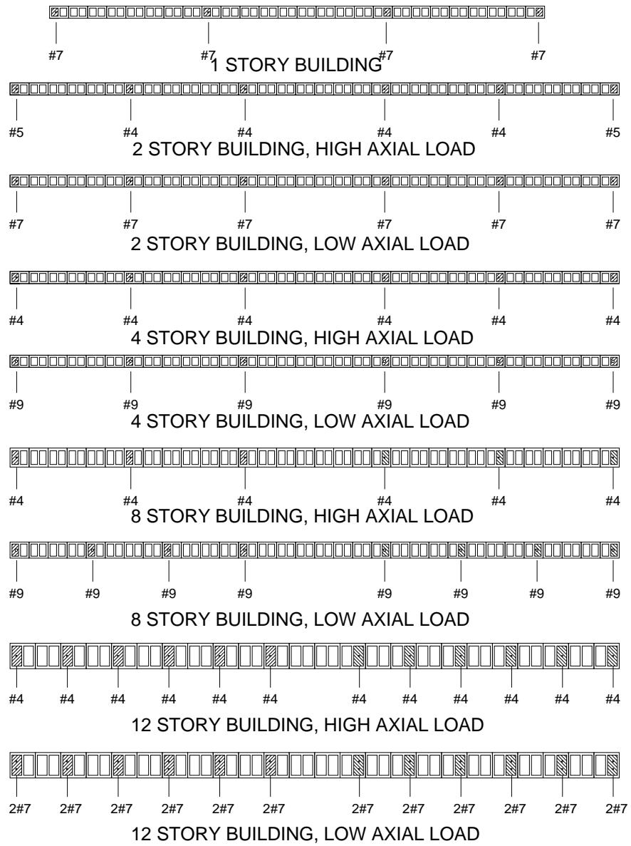
Figure A-6 Plan sections of partially grouted ordinary reinforced masonry shear walls, SDC C<sub>min</sub>.
