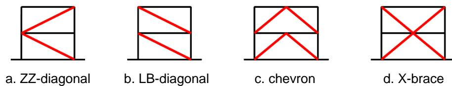
Figure 7-1      Brace configurations considered in the BRBF archetype design space.
