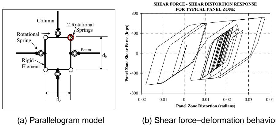
Figure 6-3 Joint panel zone model (PEER/ATC, 2010).
