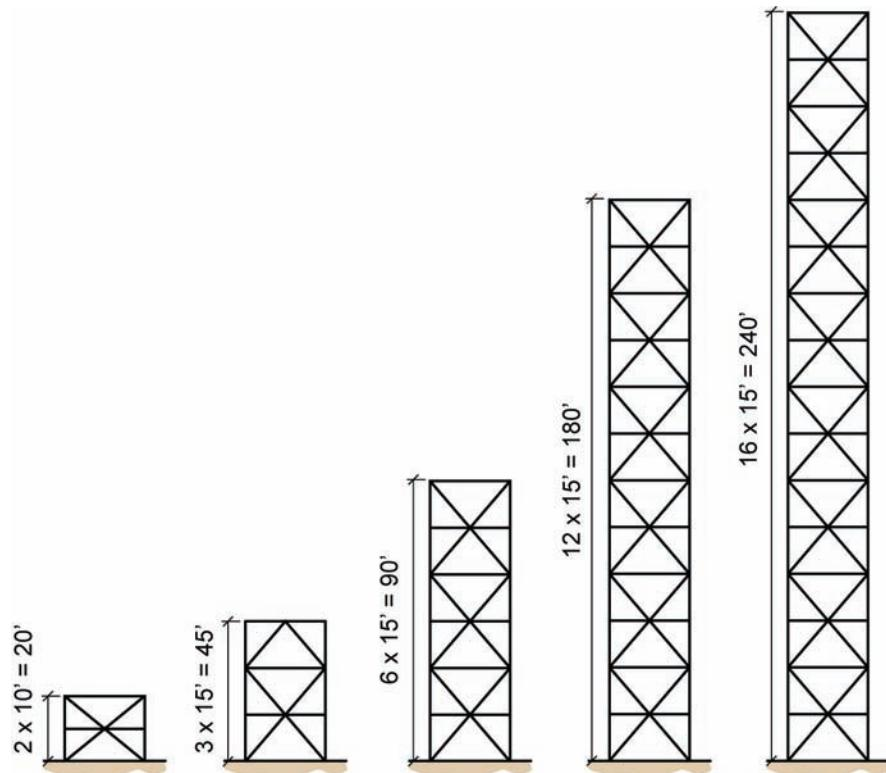
Figure 5-2      Elevation of 2-, 3-, 6-, 12-, and 16-story braced frame archetypes
