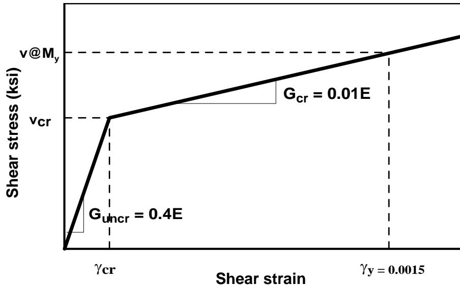
Figure B-9 Shear model with reduced shear modulus for calibration with specimen RW2.
