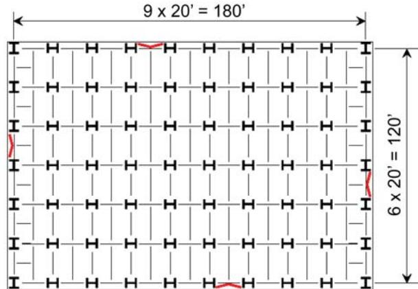
Figure C-1 Plan configuration of 2-story braced frame archetypes.
