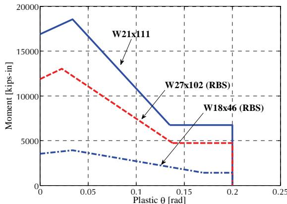
Figure 6-7 Example moment-rotation backbone curves.
