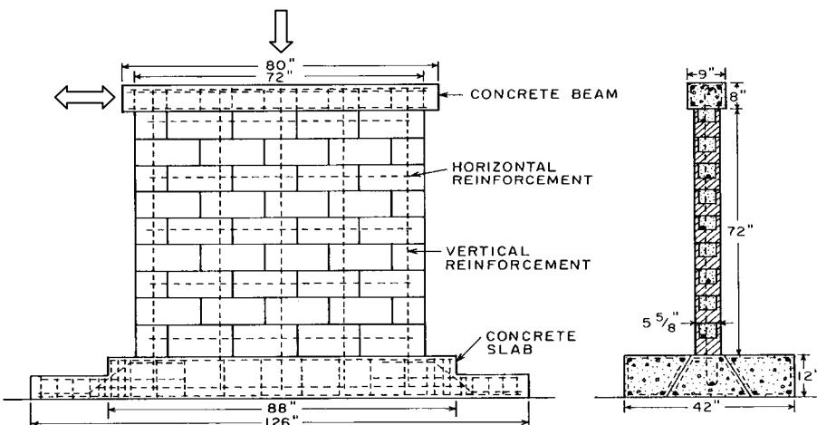
Figure 3-7 Single-story walls tested by Shing et al. (1991).
