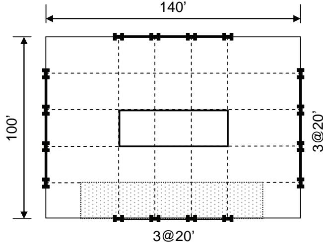
Figure 6-1      Typical plan configuration of special SMF archetypes.
